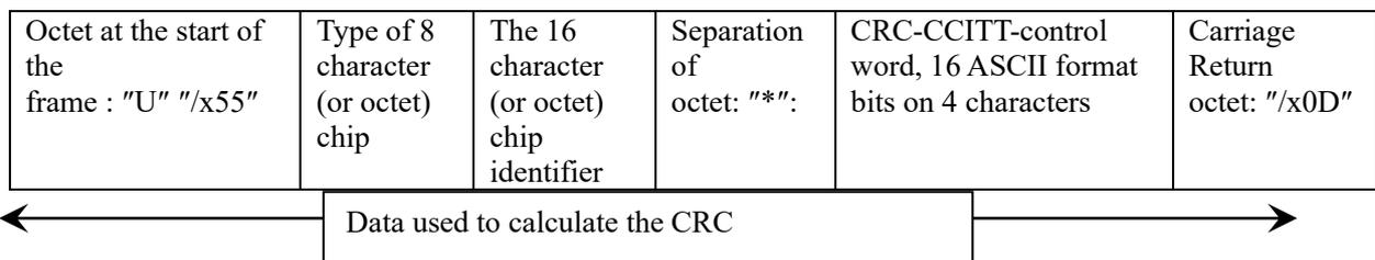
Tips: the developers of software associated with PetScan must use the head and separation characters to separate the information transmitted by PetScan, calculate a control word with the data received and compare it to the word transmitted by the PetScan to validate the information (see appendix for the CRC-CCITT-16 bit calculation algorithm)
