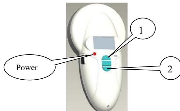
Start the V8 by holding down the Up (1) and Down(2) keys for a few seconds while pressing Power. Release the keys.
