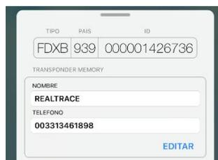
**ISO FDXB tag compatible with the possibility to write additional data A name and a phone number to datachips
